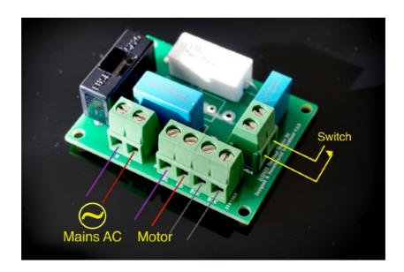
The installation is quite straightforward; the power supply has three wire sockets like shown in the picture above.
