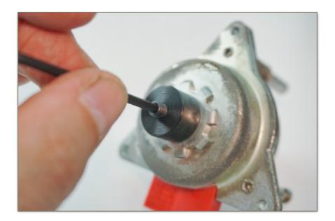
Switch on the motor and see if it rotates freely, a little friction can be expected and, since the motor spindle and the screw rotate in the same direction, the motor rotation should get rid of excess friction itself. Let the motor run for some time, ½ - 1 hour or so. Now the stopper is set. You can put a little drop of a mild adhesive on the screw to make it more resistant to involuntary movements.
